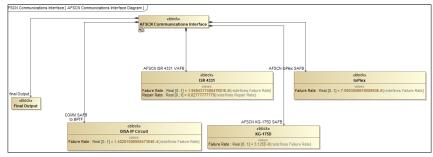
2. Transform generic SysML blocks into reliability blocks by means of inheritance
