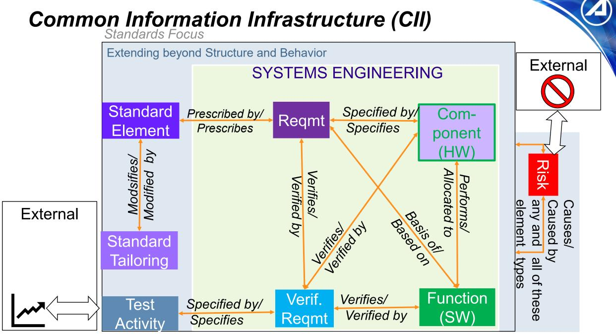
Subset of CII (not built into SysML)
