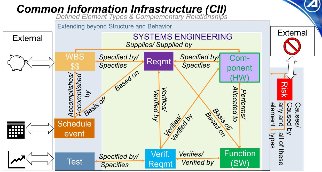
Subset of CII (not built into SysML)
